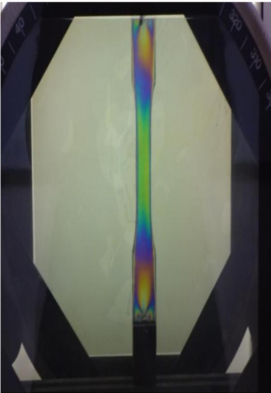
Fig.( 2) Calibration of material by tensile specimen
