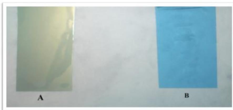
**Figure (6): Removal of gelatin from X-ray films by crude protease of *B. licheniformis* B1. The X-ray films pieces were incubated with crude protease at 30°C. for 2h. A, control (without enzyme); B, Sample treated with enzyme.**
