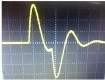
Figure 5. Output waveform of the stimulator.
