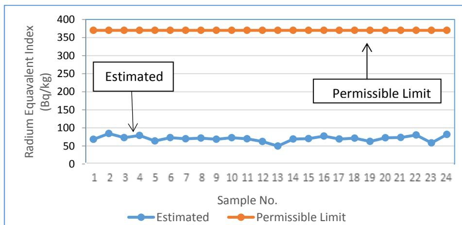
Figure (4) Comparison between the estimated radium equivalent index with the relevant permissible limit
