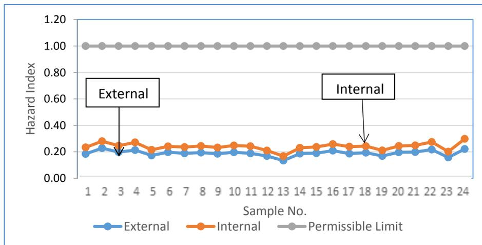
Figure (3) Comparison between the estimated internal and external hazard indices with the relevant permissible limit
