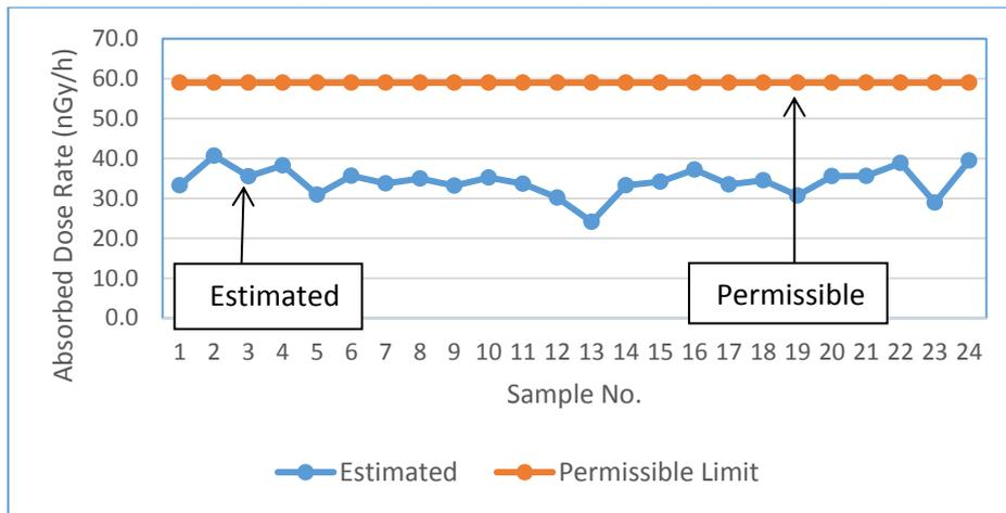
Figure (2) Comparison between the estimated absorbed dose rate with the relevant permissible limit
