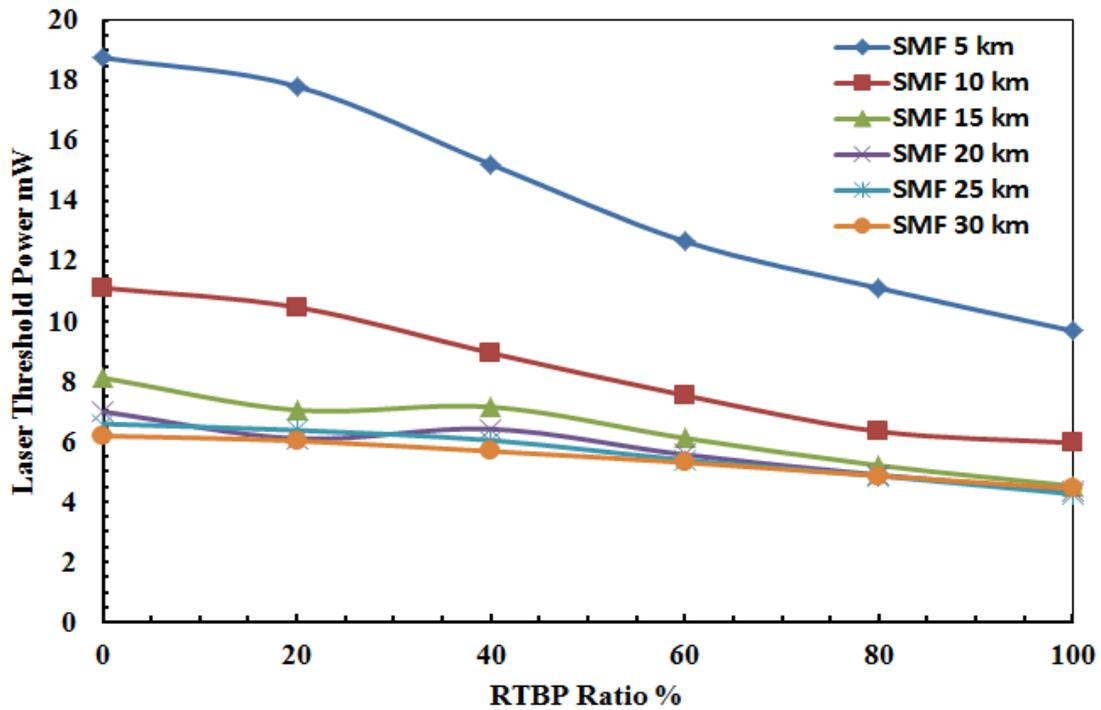
Figure 4: Laser threshold power versus the RTBP ratio %.
